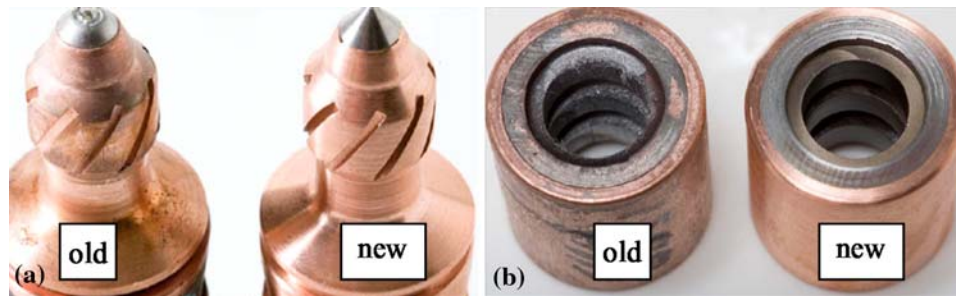
Fig. 14 (a) Cathode after 200 h run and (b) anode after 1500 h run
